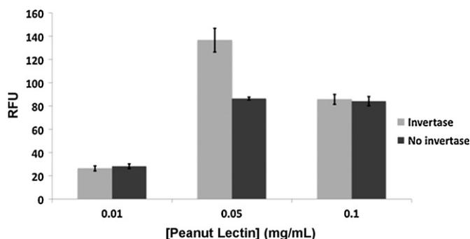
**Fig. 4.** Plot for the dependence of fluorescence signals on peanut lectin (PNA) concentration in the presence (gray) and absence (black) of 25  $\mu\text{g}/\text{mL}$  invertase. Error bars indicate the standard deviation of the repetitive measurements ( $n=4$ ).
